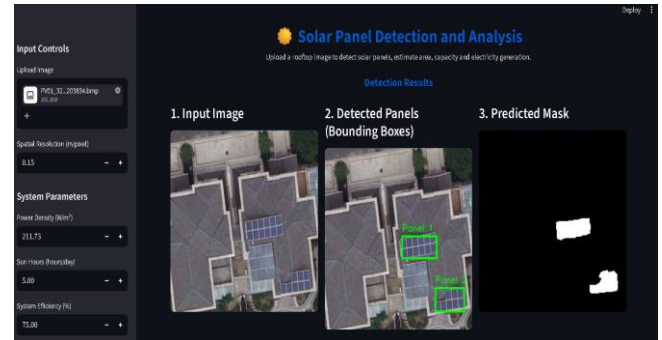
Figure 2: Streamlit user interface for rooftop PV detection and solar analysis
