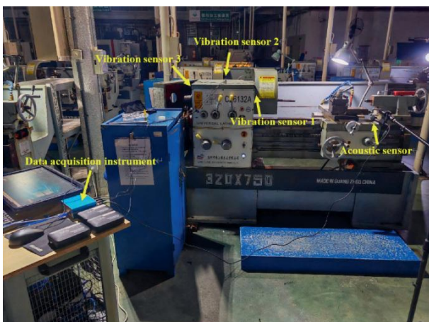
Figure 3: Sensor and embedded system architecture
